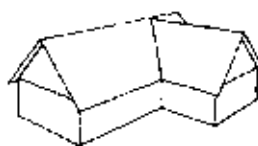
Corner roof house
